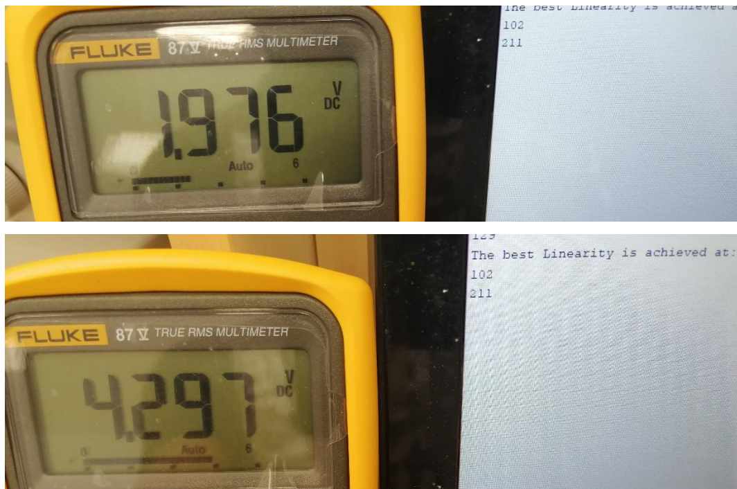
Figure 6.17 The output voltage vs the displayed number of bits
